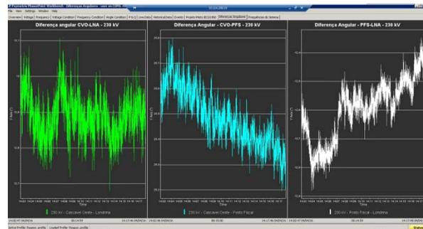
Figure 6. Customized view showing angle differences that are of interest for real-time operation.
