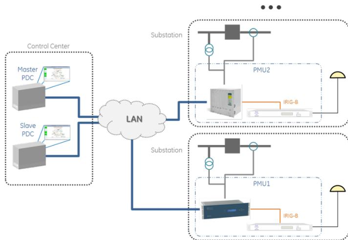
Figure 3. COPEL's WAMS communication architecture.
