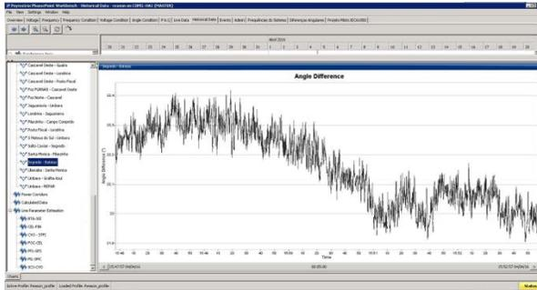
Figure 7. Angle difference from Segredo to Bateias 525 kV busbars.
