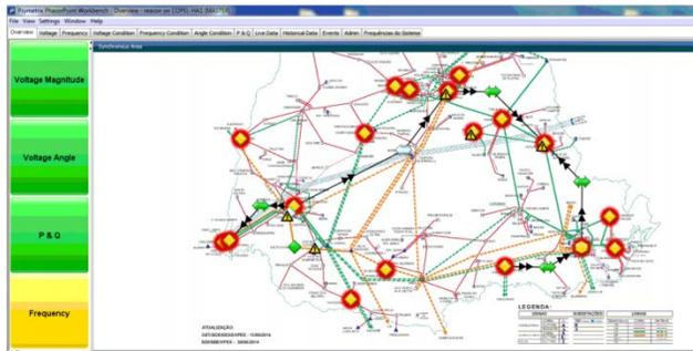
Figure 9. Main software screen indicating that the system was at alert frequency condition.
