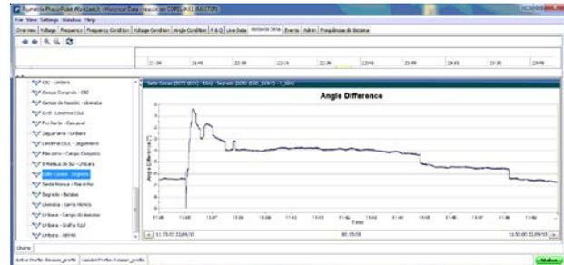
Figure 16. Angle difference between Salto Caxias and Segredo busbars at full disturbance period.
