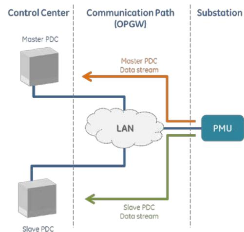
Figure 4. Communication strategy used for redundancy of data.
