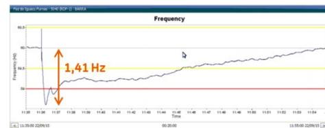
Figure 14. Frequency behavior at 525 kV CVO busbar at disturbance period.
