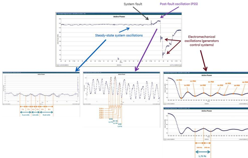
Figure 17. Power oscillations verified at a transmission line connected to GPS 230 kV busbar.
