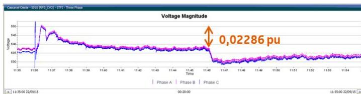
Figure 13. Voltage magnitude behavior at 525 kV CVO busbar at disturbance period.
