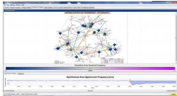
Figure 10. Frequency condition tab displaying information about frequency in real time at disturbance period.
