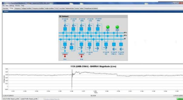
Figure 11. Voltage magnitude behavior at the disturbance in Umbará 230 kV substation.
