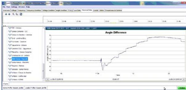
Figure 15. Angle difference between Salto Caxias and Segredo busbars in the first seconds of the disturbance.
