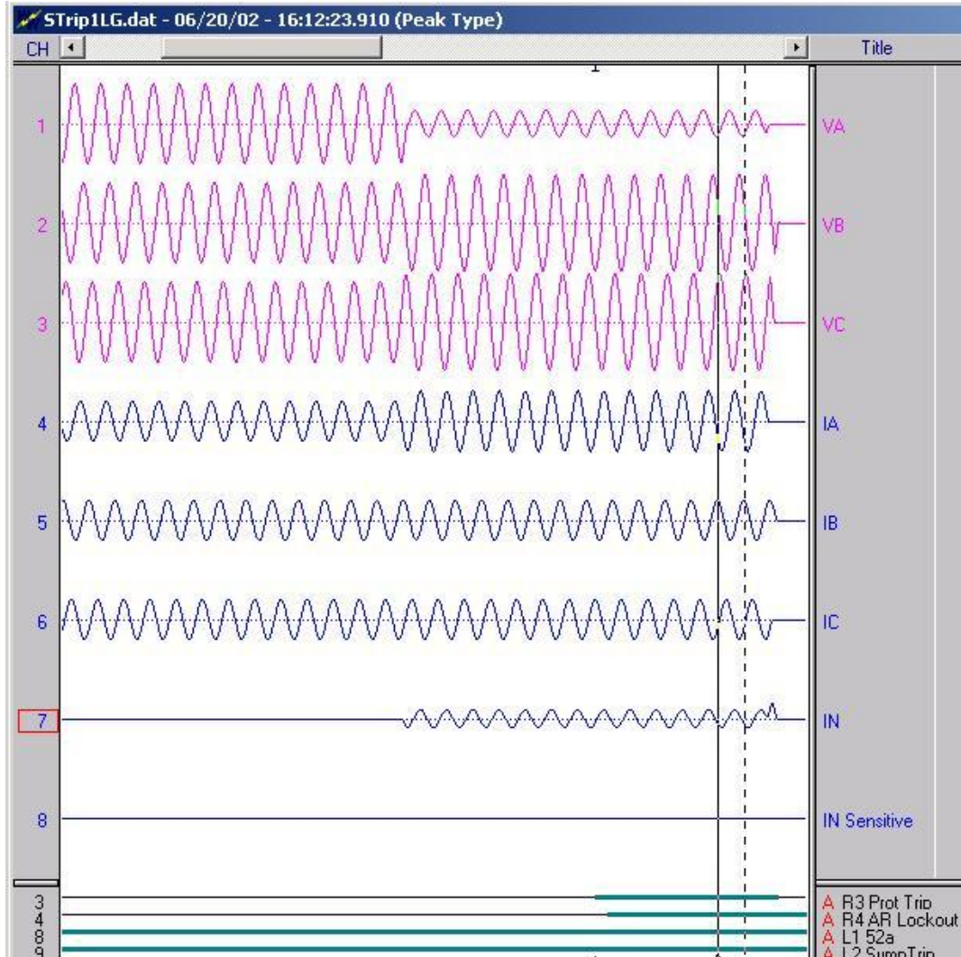
Fig. 6 Waveform record including state change information
