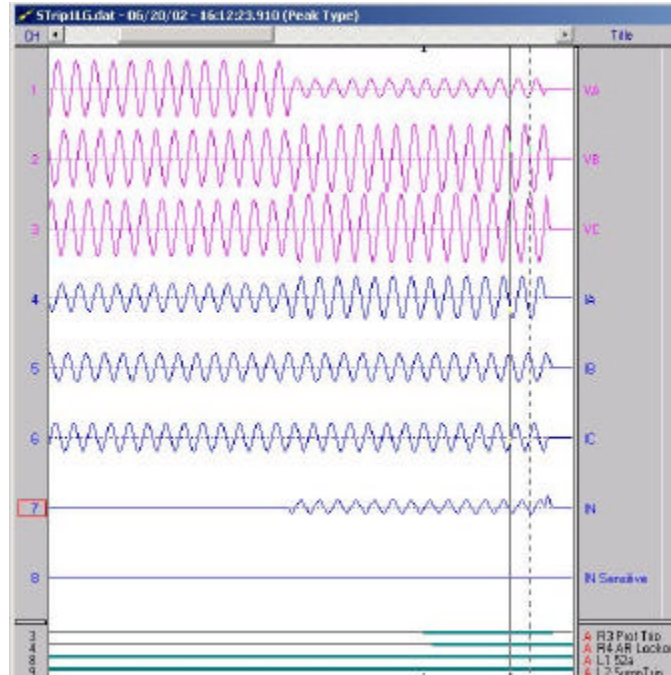
Fig. 2 Waveform record including state change information
