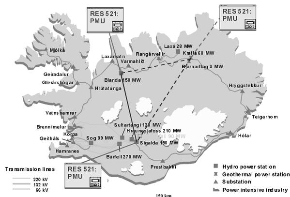
**Figure 1:** The Icelandic power system with a 132 kV ring network and a meshed 220 kV network with the majority of the power plants in the south and Reykjavik in the southwest. PMU locations shown are Blanda (north), Krafla (northeast – to be installed) and Sigalda (south).
