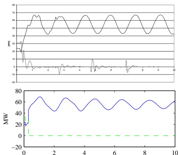
**Figure 2:** Recording (top) and simulation (bottom) of disturbance 2001-02-16. Plots use the same scale and show ten seconds of line flow west and east of Krafla, when the latter is faulted and tripped together with one Blanda unit.
