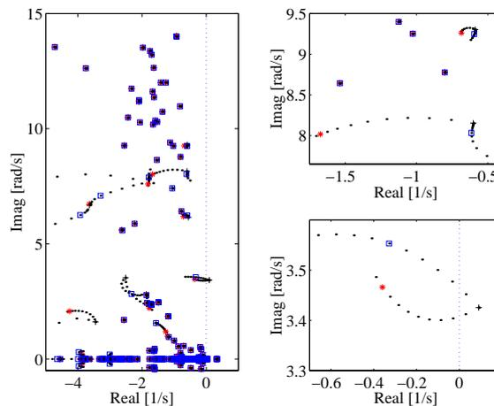
**Figure 7:** Root locus plots with gain ranging from zero (+) to 20 in steps of 2 for case 4 with overview (left) and details (right). Selected gains are indicated for local PSS (\*) and wide-area PSS (square).
