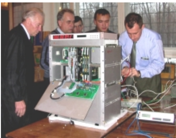
Fig. 2. Digital fault recorder BEN 5000
