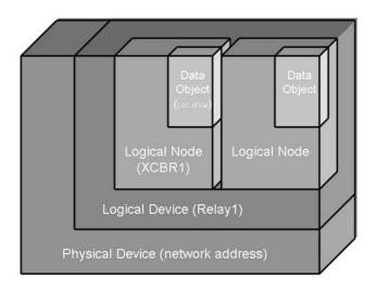
By developing models using common naming conventions shared by all devices participating in an IEC 61850 based system, data may be easily exchanged throughout the system without the need of specifically identifying items such as: device driver, physical wiring between devices, data register, and network address.
