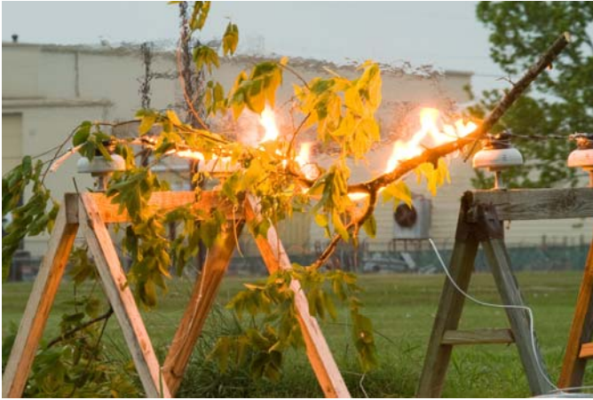
Fig. 8. Arcing branch, Experiment 3.
