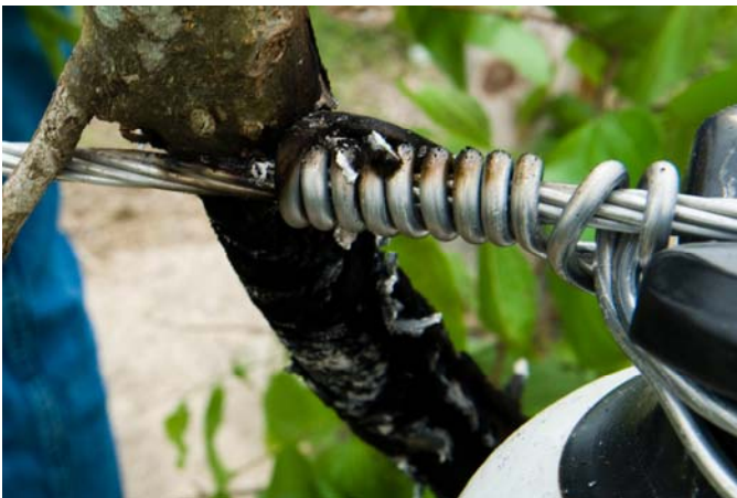
Fig. 10. Main branch remains on conductor, Experiment 3.
