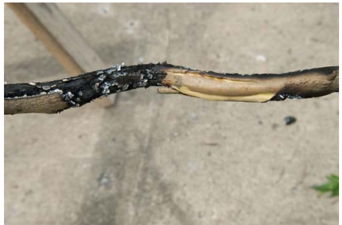
Fig. 4. Damage to branch, mid-branch after Experiment 1.
