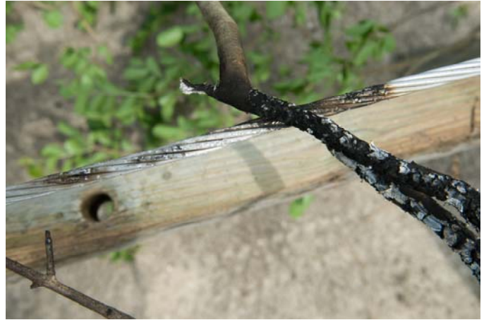
Fig. 2. Damage to branch and phase conductor after Experiment 1.
