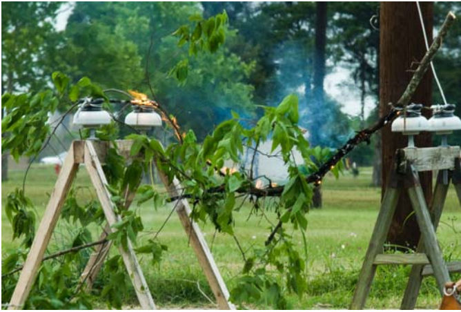
Fig. 9. Burned-through branch immediately after final arc burst, Experiment 3
