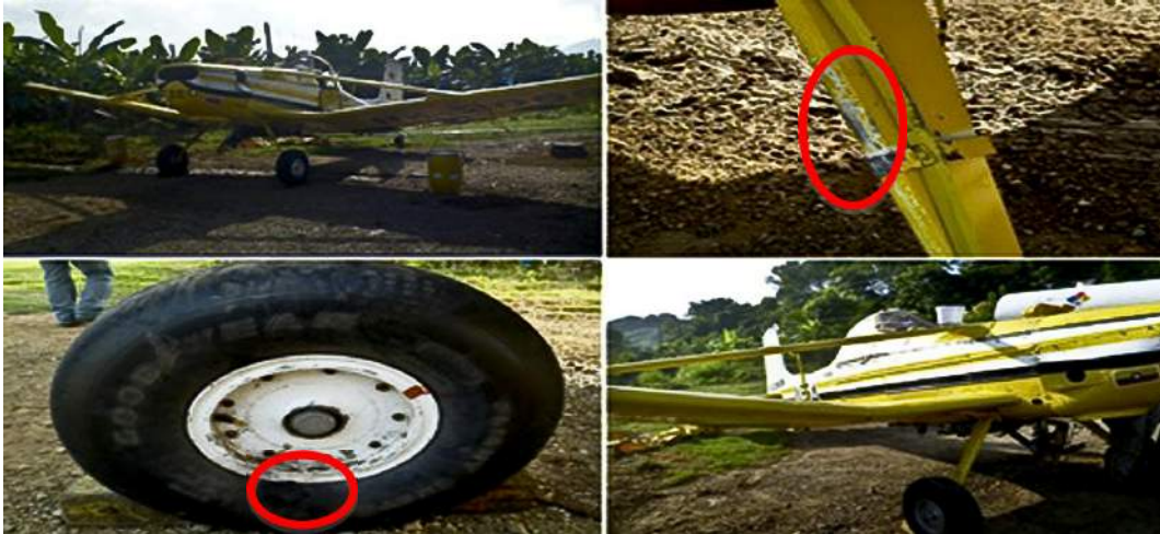
Figure 5. Light aircraft used for aerial fumigation that caused the fault in circuits LN-814 and LN-815.
