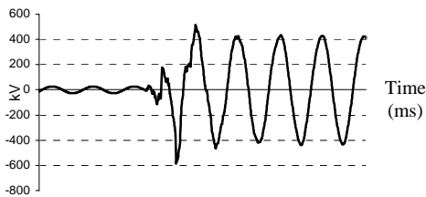
Fig 12- Phase b Voltage Measured by the Voltage Divider
