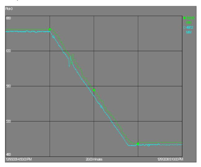
This example shows comparison of EMS data (6 second scan rate) and Phase 1 Analog Telemetry Data Acquisition System for shutdown of a DC link. Notice the stair-step effect in the 6 second scan data. Also, the transient is shown nicely in Phase 1 Analog Telemetry Data Acquisition System plot, but obscured in 6 second data. The transient is irrelevant and the cause is unknown.
