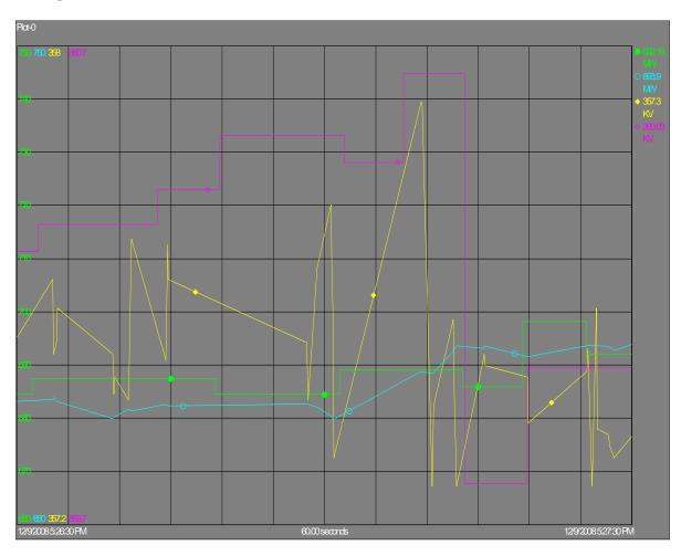
This example shows comparison of EMS data (6 second scan rate) and Phase 1 Analog Telemetry Data Acquisition System for shutdown of a DC transmission link. The Phase 1 Analog Telemetry Data Acquisition System plots are yellow and light blue and in this case are far more useful than the EMS data.
