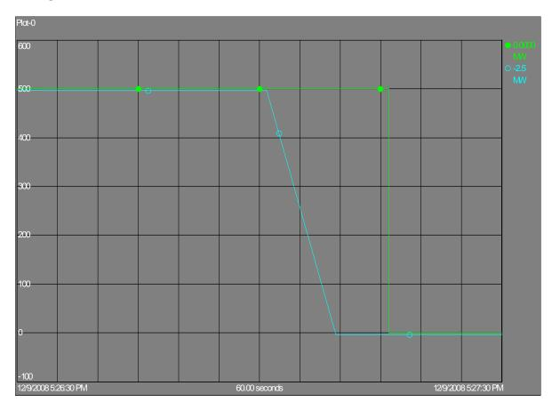
This example shows comparison of the EMS data (6 second scan rate) and Phase 1 Analog Telemetry Data Acquisition System for shutdown of a DC link. Notice that the slower scan rate and filters in the green plot make this appear to be a step change in MW, while Phase 1 Analog Telemetry Data Acquisition System reveals the MW change to be a fast ramp.
