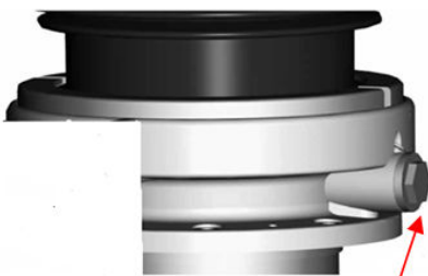
Tap point on lower part of bushing
