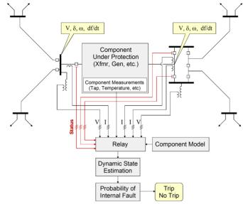
Figure 2: Illustration of Settingless Component Protection Scheme
