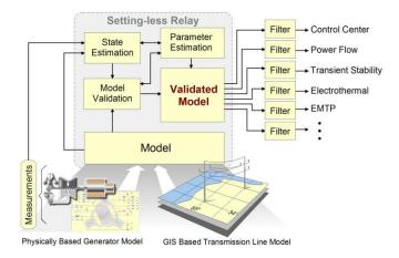
Figure 6: Illustration of Settingless Protection Logic
