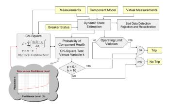
Figure 3: Illustration of Settingless Protection Logic
