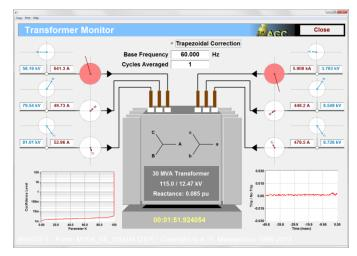
Figure 5: Visualization of Transformer Setting-Less Protection
