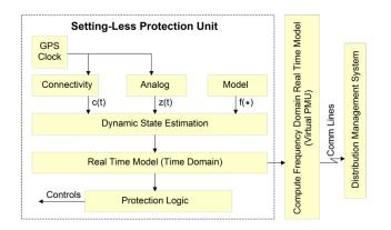
Figure 7: Functional Diagram of Setting-less Protection Unit
