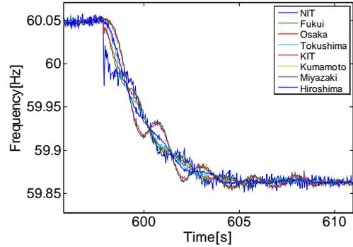
Fig. 10. Frequency under generator trip.
