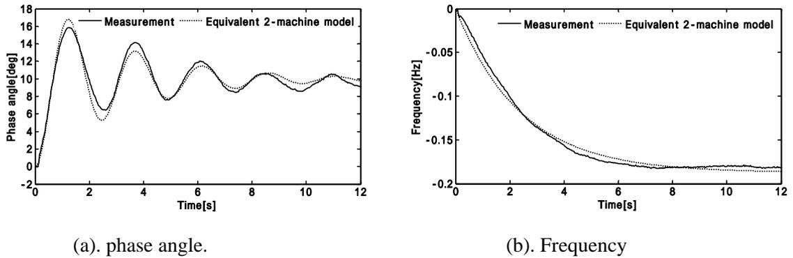
Fig. 15. Phase angle and frequency transient after fault.
