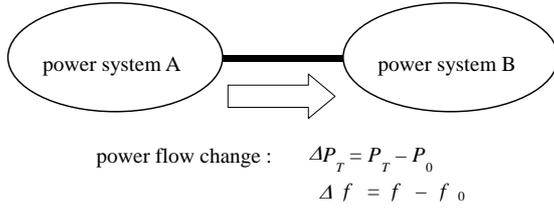
Fig. 13. Model of two interconnected power systems.
