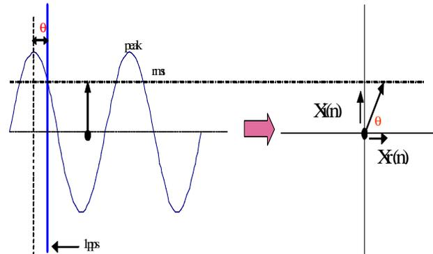
**Figure 1: Phasor measurement in relation to the common reference value:**
