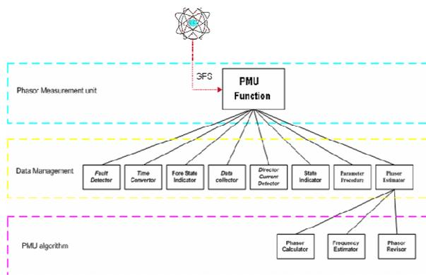
As shown above, the PMU data are synchronized with UTC time from a GPS receiver with accuracy of <1microsecond and captured at a rate of 10,12,15,20,30 and 60 frames per second at 60 Hz, and can be used to support:
