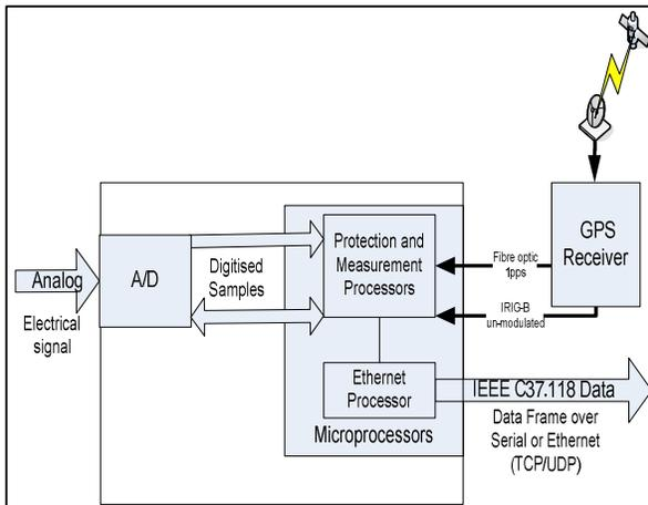
**Figure 2: Phasor measurement architecture**
