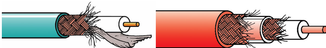
Figure 9: coaxial cable (left) & triaxial cable (right)
