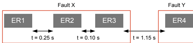
Fig. 4 Example of distribution feeder event reports showing time-based grouping with a one-second grouping threshold
