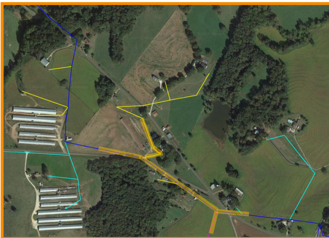
Fig. 6 Subsection of Oakway substation Feeder 6 with fault location range overlay
