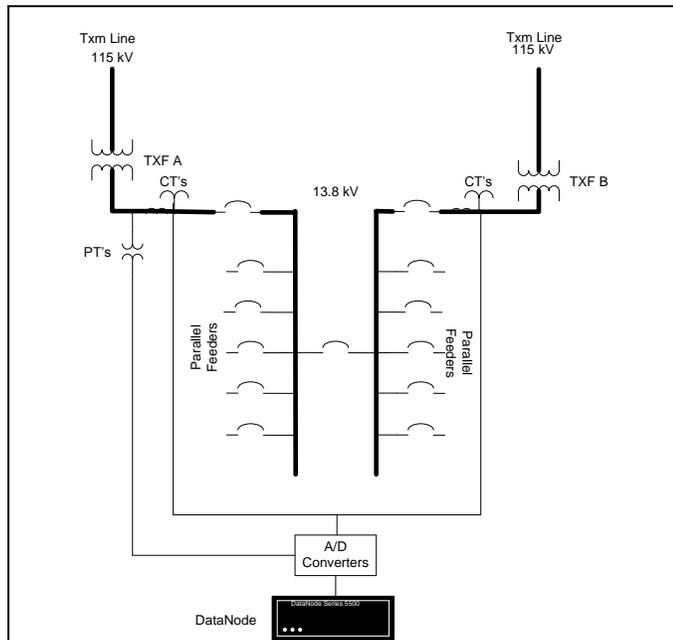
**Figure 1: Typical Connection of Power Quality Monitor at UI Company**
