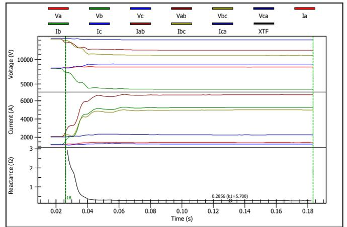
**Figure 5: Calculation of Reactance-to-Fault for SLG Fault in Figure 2**
