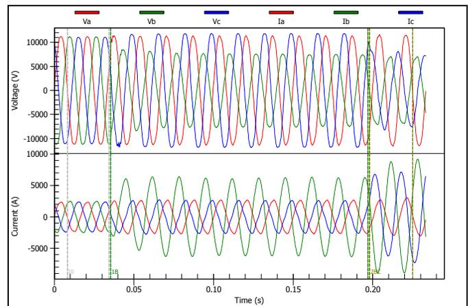
**Figure 3: Example SLG Fault on a UI Company Distribution Line that Evolves to Become Two-Phase**
