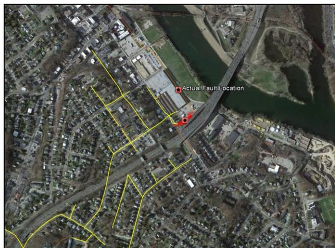
**Figure 7: Example One-Line Diagram Showing Estimated Fault Locations and Actual Location Displayed with Aerial Map Data for SLG Fault in Figure 2**
