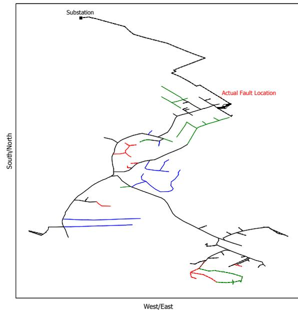
**Figure 6: Example One-Line Diagram Showing Estimated Fault Locations and Actual Location with Coordinates for SLG Fault in Figure 2**
