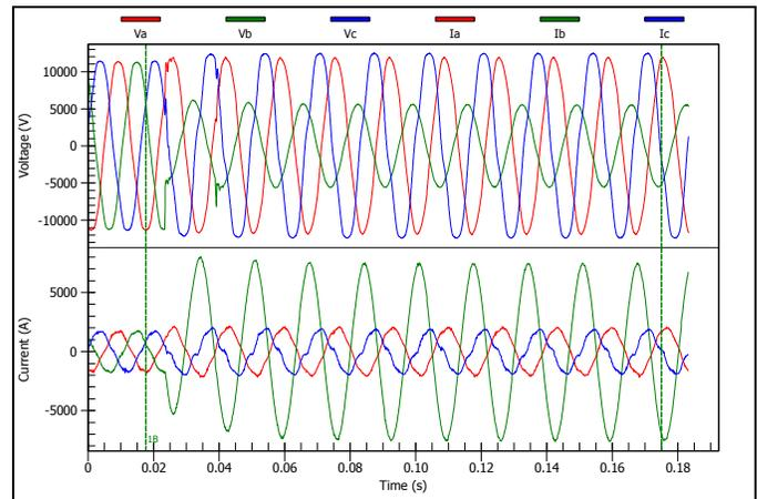
**Figure 2: Example of a SLG fault on a UI Company distribution feeder**
