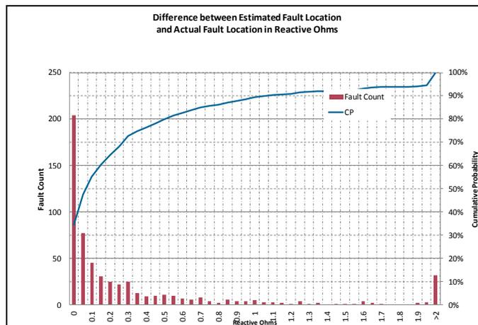
Figure 11: Fault Location Estimation Accuracy
