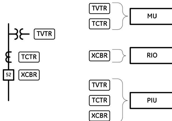
Figure 9: Process bus devices
