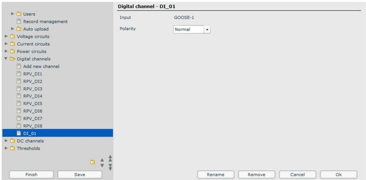
Figure 16: GOOSE digital channel configuration
