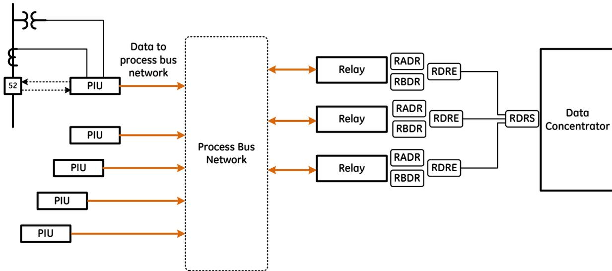
Figure 12: Virtual recording using process bus
