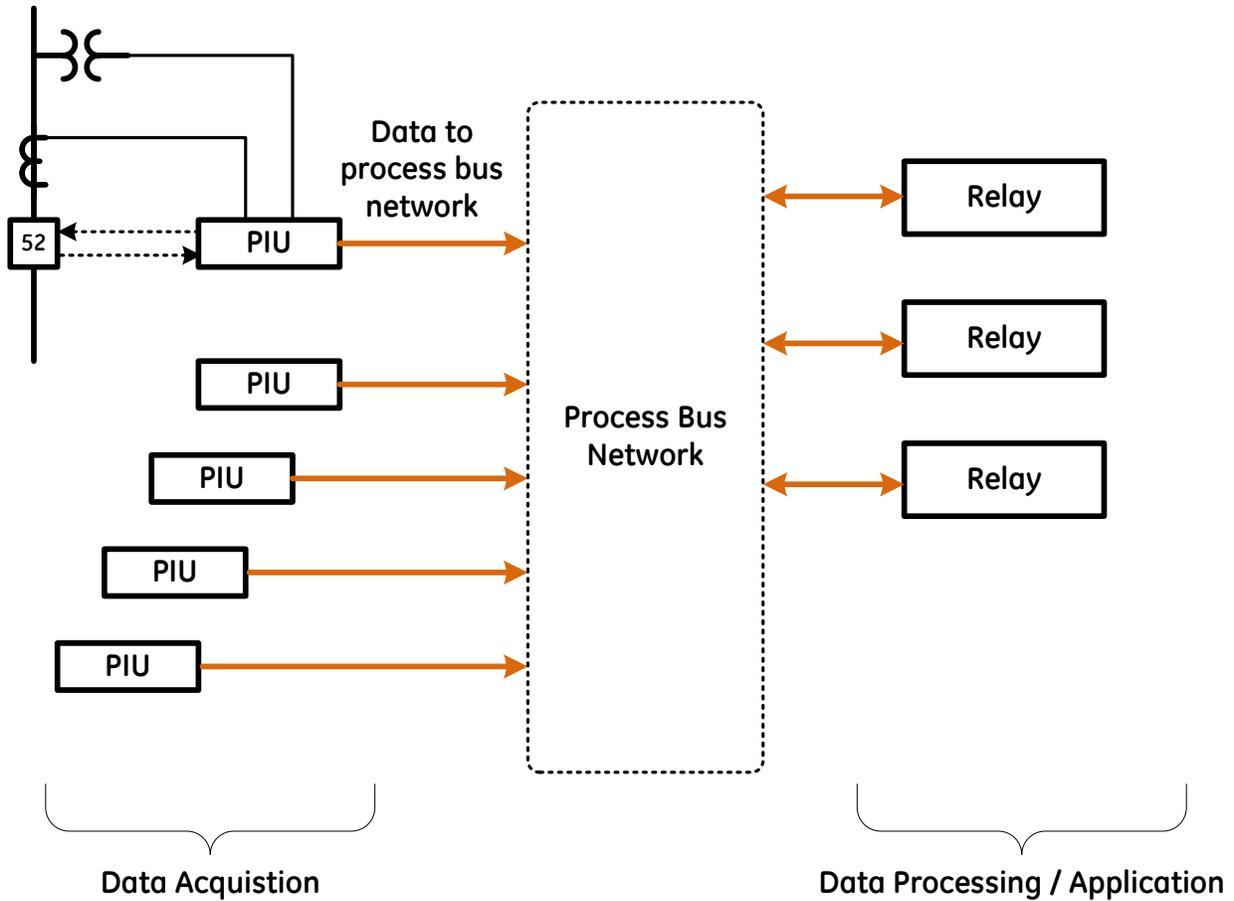
Figure 11: Process bus system
