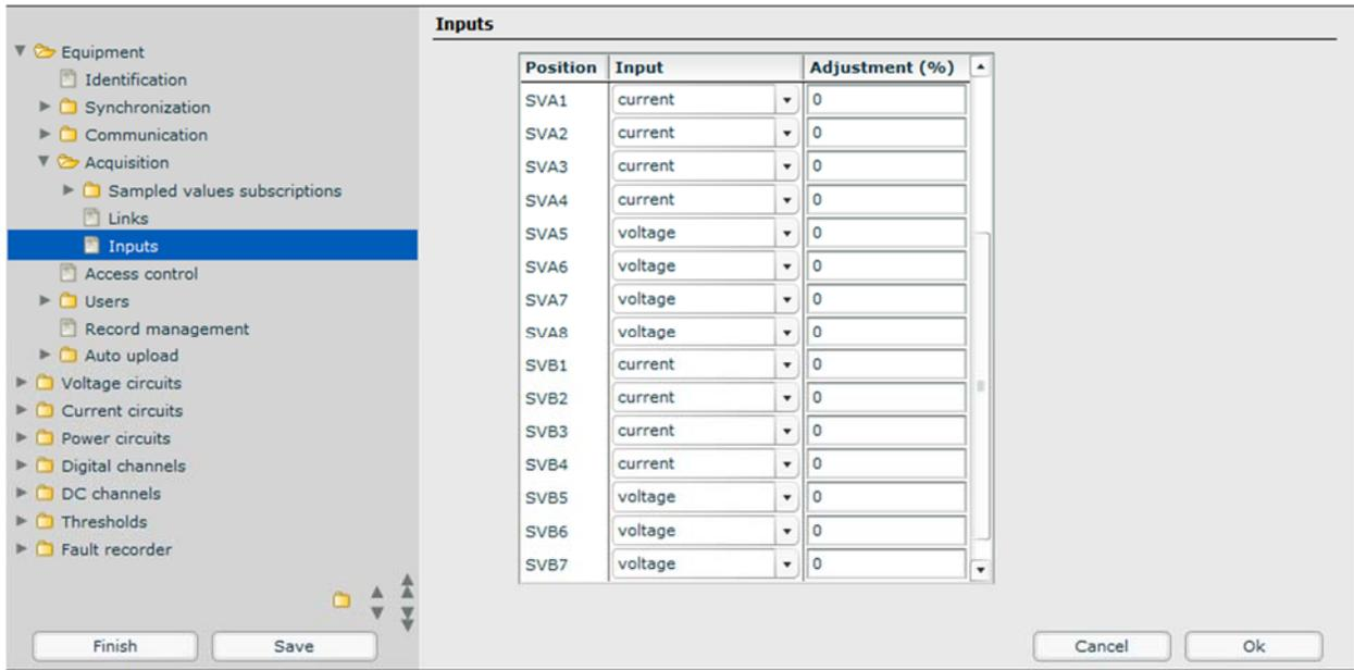
Figure 15: SV analog channel configuration
