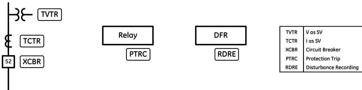
Figure 6: Functional modeling of DFR arrangement
