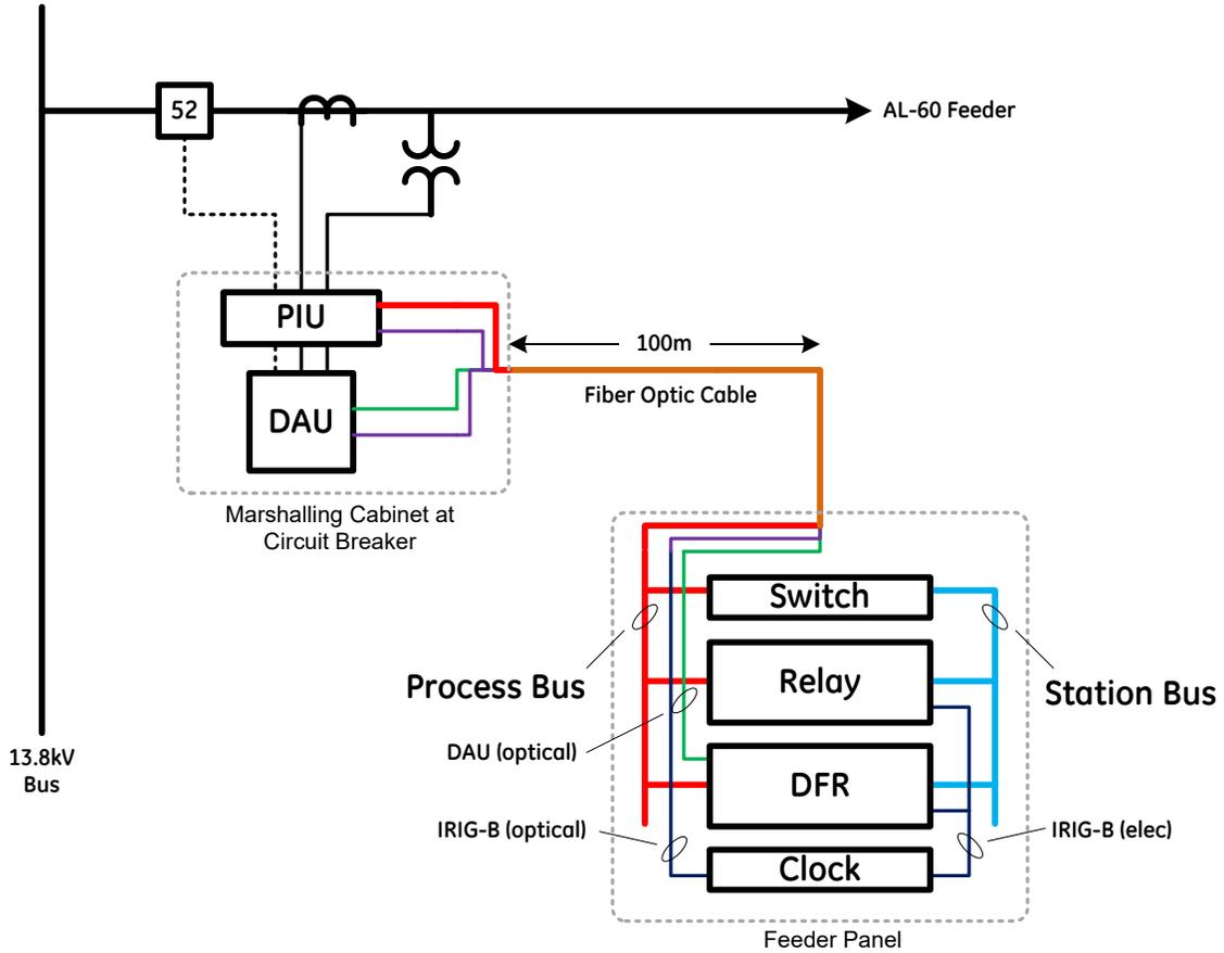
**Figure 18: CTEP Embu-Guaça Substation dedicated DFR over process bus**
