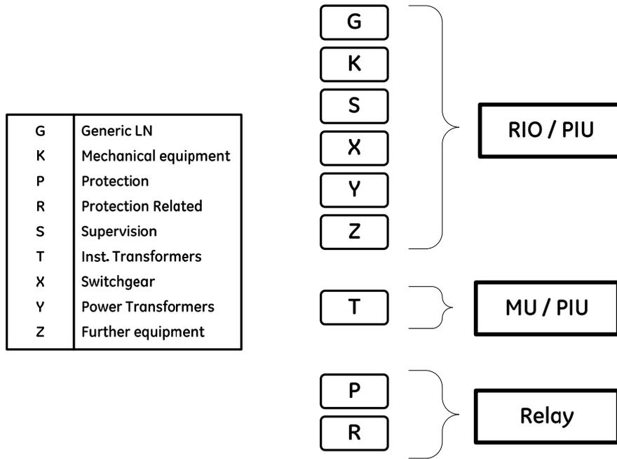
Figure 10: Possible source devices for data
