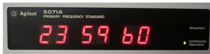
Figure 5: Leap second displayed on a Caesium Beam Tube frequency standard
