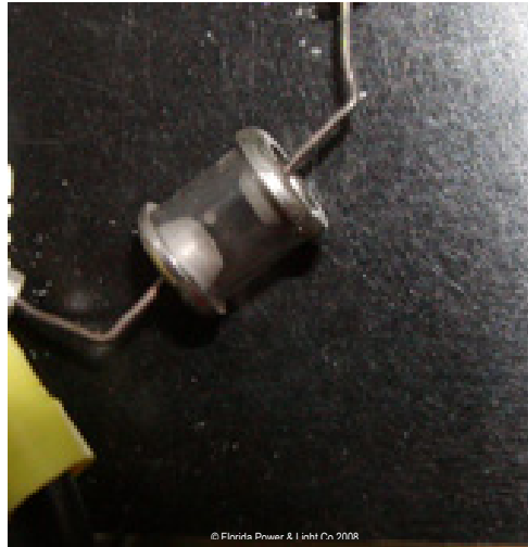
Figure 8 - Closer view of non-adjustable Gaps
