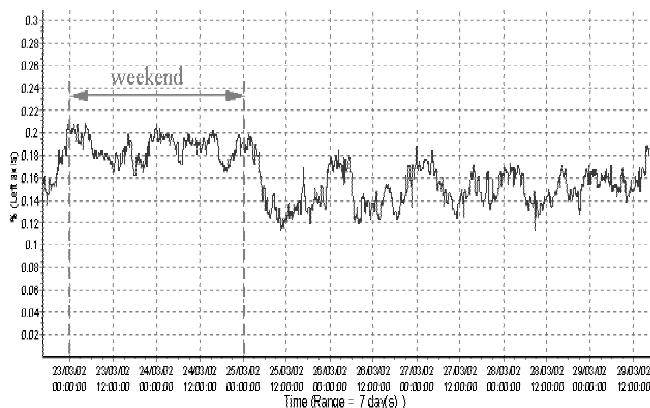
Fig. 23. Typical change of the k_a factor during the example week (WANDA)
