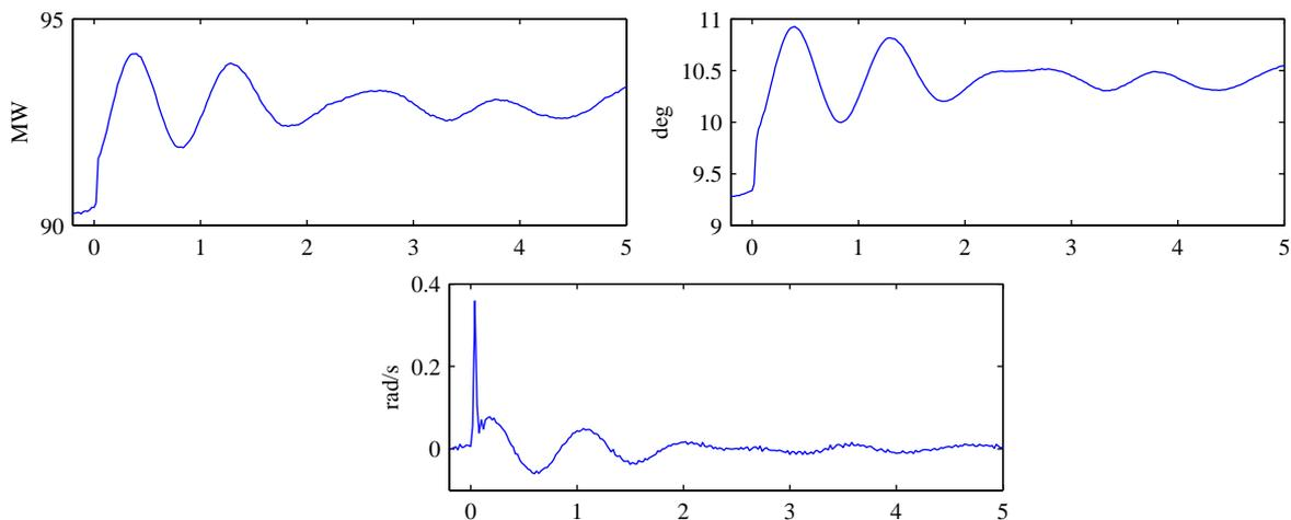
**Figure 5: Recording from closing of line between Blanda and Krafla showing line flow east of Blanda (left) phase angle difference Blanda-Sigalda (right) and frequency difference Blanda-Sigalda (bottom).**
