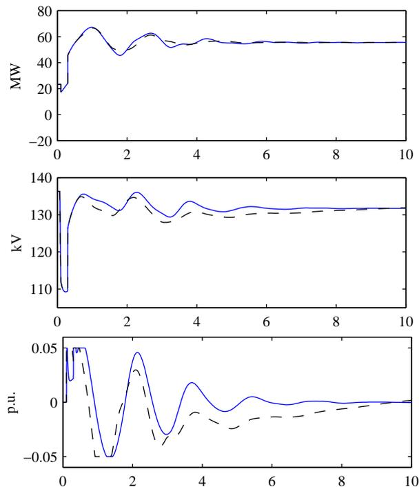
**Figure 8:** Simulation of 2001-02-16 disturbance with speed-input (dashed) and with wide-area PSS (solid). Plots show real power on line west of Krafla (top), voltage near Krafla (center) and PSS output (bottom).
