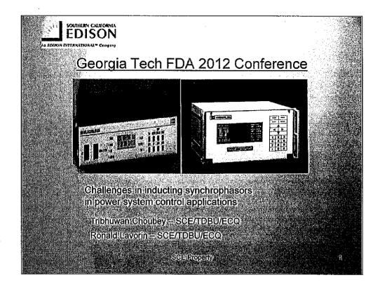
Phasor representations of voltages and currents at key locations throughout the power system define the state of the network. The Macrodyne Model 1690 Phasor Measurement Unit (PMU) provides instant access to this information providing new opportunities to understand and improve the performance of today's power systems.
