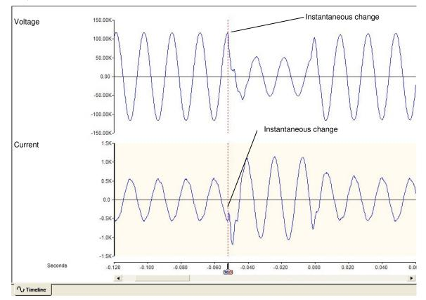
disturbances, and load fluctuations will help determine appropriate triggers to use to securely record a power system fault.
