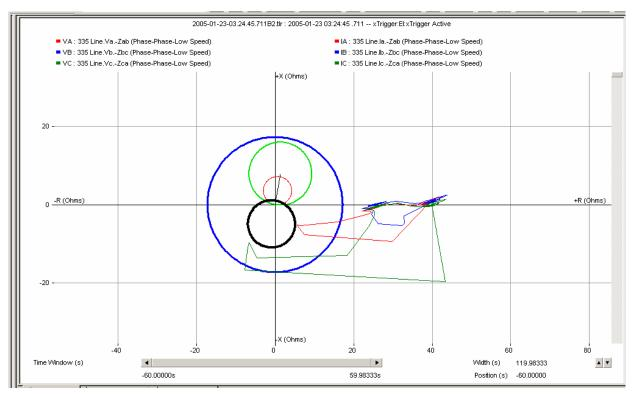
Figure 9: Impedance trigger for protection system verification
