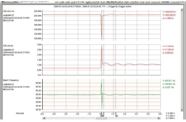
Figure 6: Voltage and Current quantities from power equipment fault
