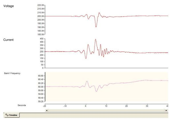
Figure 2: Power system fault (swing) record
