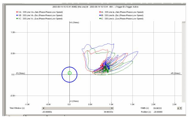
Figure 7: Impedance trigger for power swing event
