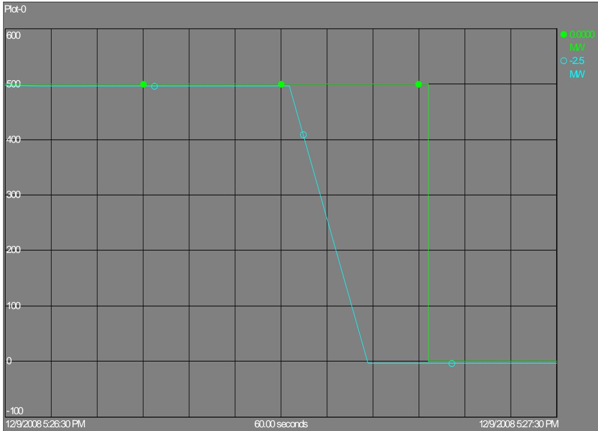
This example shows comparison of the EMS data (6 second scan rate) and Phase 1 Analog Telemetry Data Acquisition System for shutdown of a DC link. Notice that the slower scan rate and filters in the green plot make this appear to be a step change in MW, while Phase 1 Analog Telemetry Data Acquisition System reveals the MW change to be a fast ramp.
