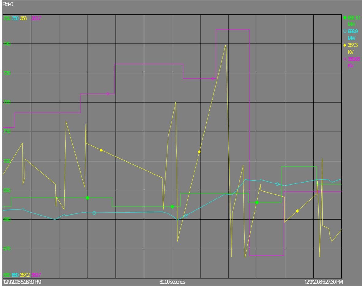
This example shows comparison of EMS data (6 second scan rate) and Phase 1 Analog Telemetry Data Acquisition System for shutdown of a DC transmission link. The Phase 1 Analog Telemetry Data Acquisition System plots are yellow and light blue and in this case are far more useful than the EMS data.
