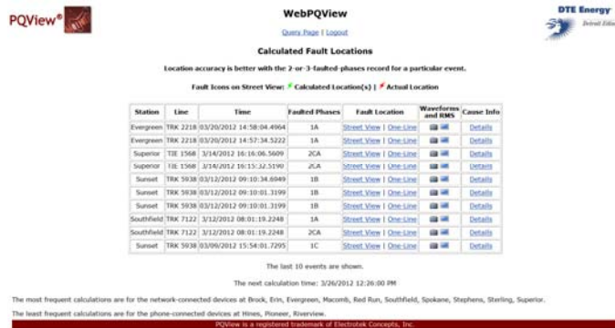
Figure 9: Web Table Display of Estimated Fault Locations
