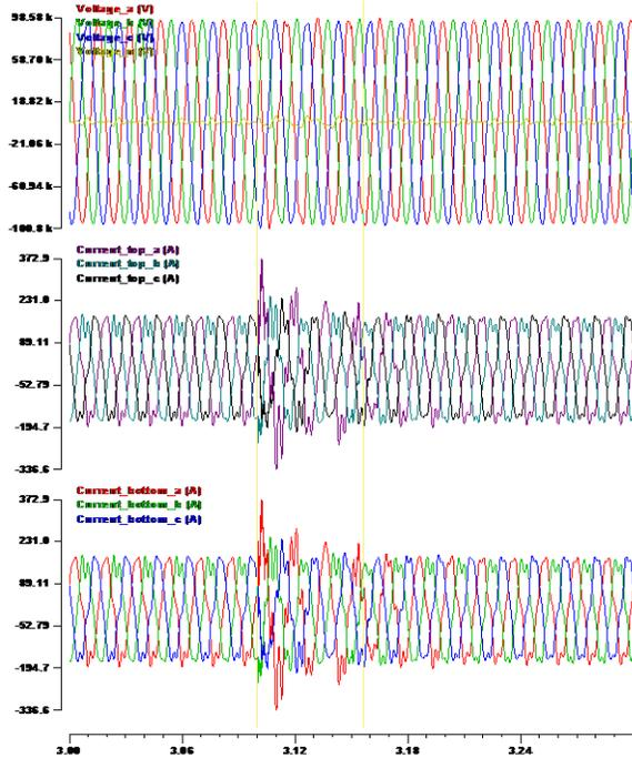
Figure 11. Simulation Results for an Internal Fault Event: Measured Signals at the Capacitor Bank
