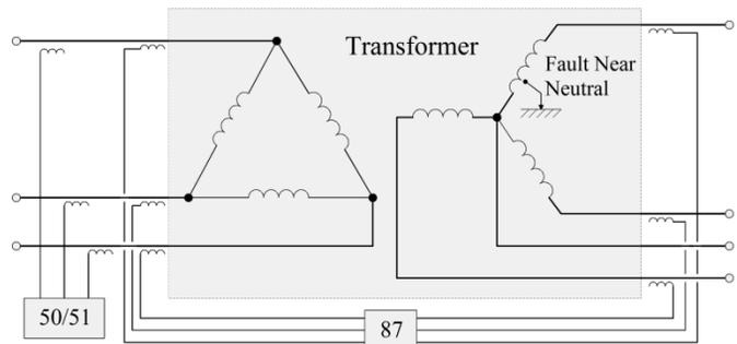
Figure 1. Transformer Overcurrent and Differential Protection
