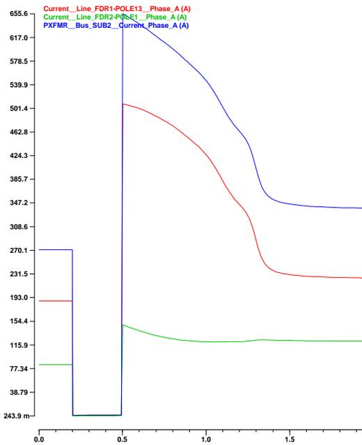
Figure 2. Feeder Overcurrent During Fault-induced Delayed Voltage Recovery
