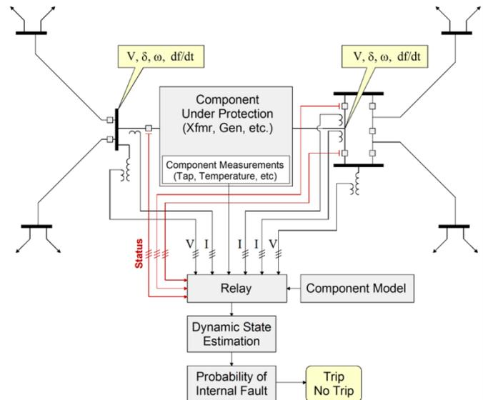
Figure 3. Illustration of Settingless Component Protection Scheme
