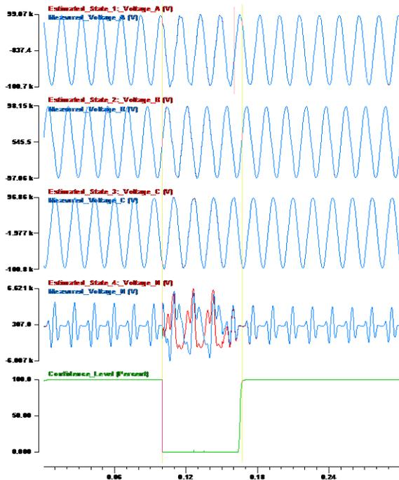
Figure 12. Internal Fault Event: Measured and Estimated Values, Confidence Level
