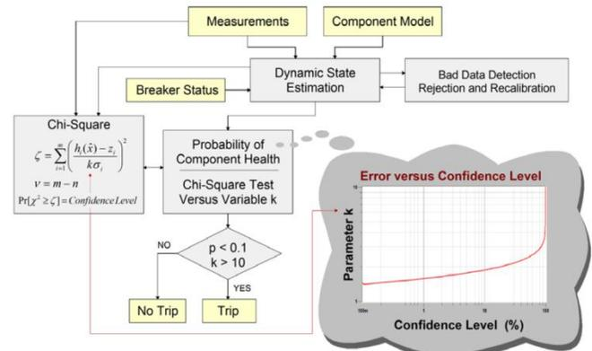
Figure 4. Illustration of Settingless Protection Logic
