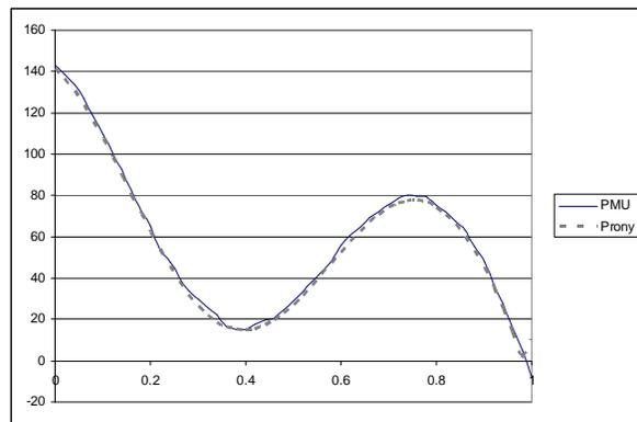
**Figure 11: PMU output and Prony fit**
