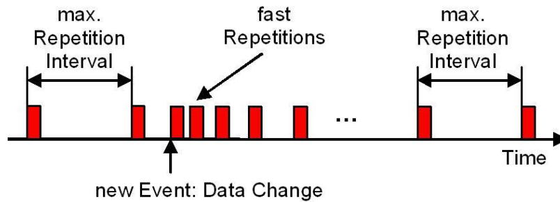
Fig. 2 GOOSE repetition mechanism
