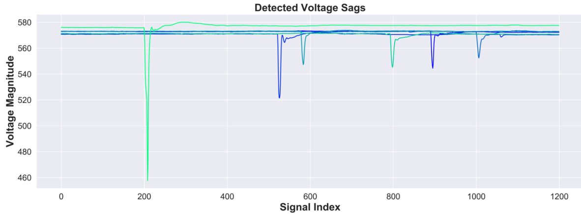
Figure 7 - Visualization showing the actual phasor magnitude data for each detected voltage sag.
