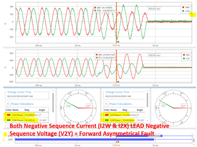
Figure 5d: V2 and I2 Relationship at Substation D Line # E1 from relay Event Record
