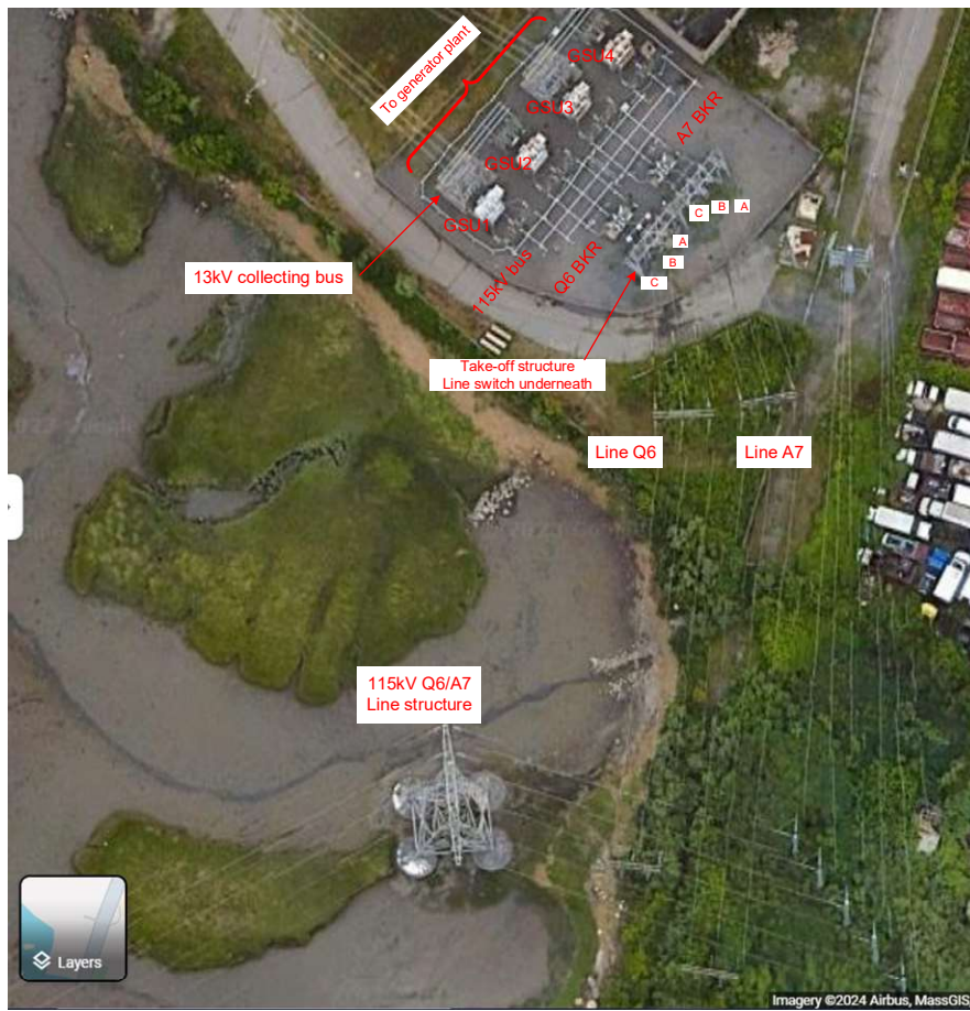
Figure 8: A bird view of generation facility yard by courtesy of Google map
