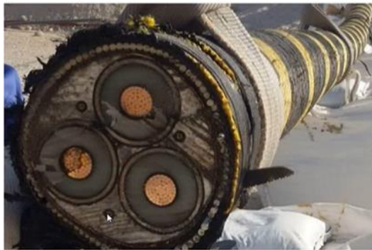
Figure 2: Cross-section of Similar 72kV Undersea Power Cable
