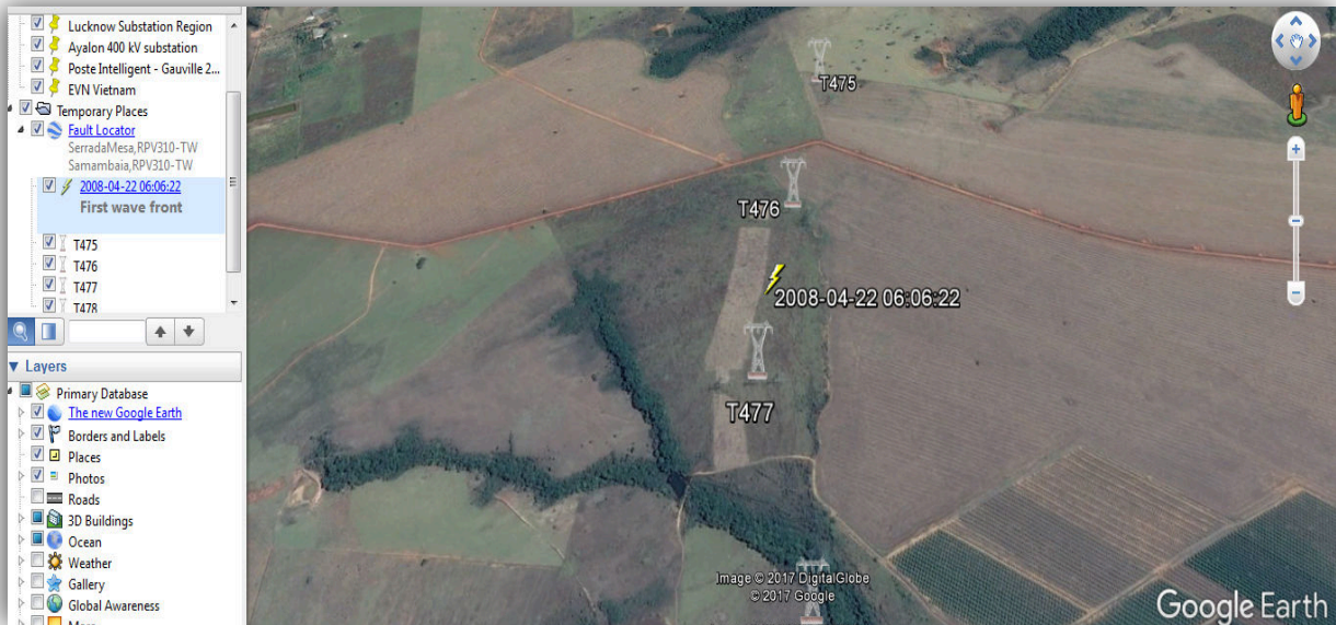
Figure 7 – TW Fault location integrated with Google Earth
