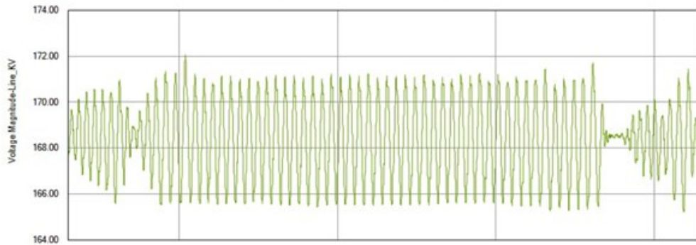
Fig. 13. Example voltage oscillation resulting from MVAR swings
