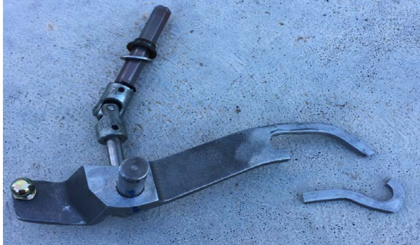
Figure 13 CB 572 Broken Linkage Lever
