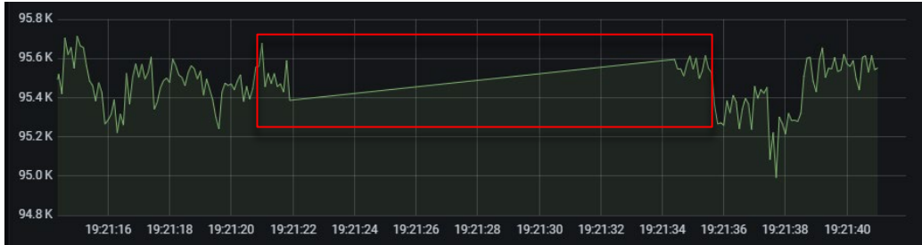
Fig. 1. Substation A - Voltage Synchrophasor Plot with Missing Data Outlined in Red
