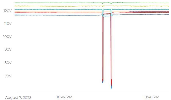
Figure 13 - Voltage Sag at 10:48 pm
