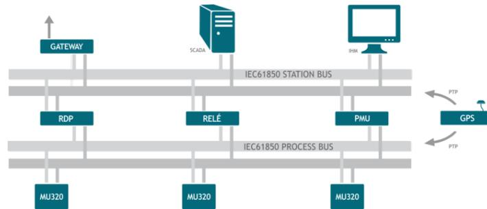
FIGURE 1 – Process Bus and Station Bus
