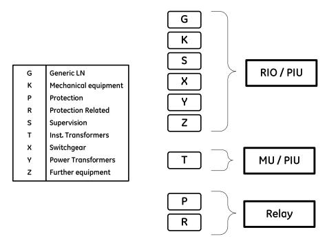
Figure 10: Possible source devices for data
