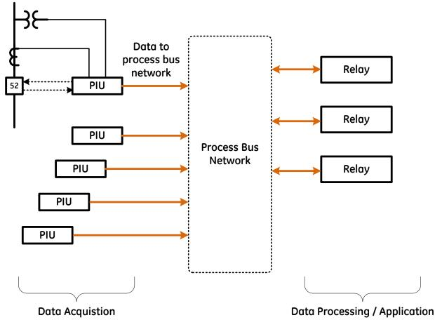
Figure 11: Process bus system
