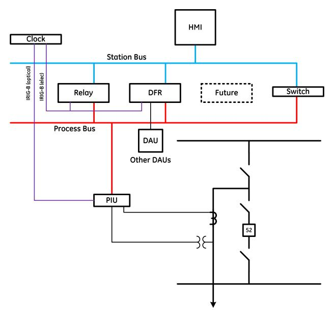
Figure 17: Electrosul Palhoça Substation dedicated DFR over process bus
