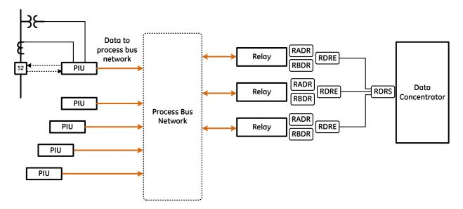
Figure 12: Virtual recording using process bus
