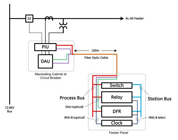
Figure 18: CTEEP Embu-Guaça Substation dedicated DFR over process bus
