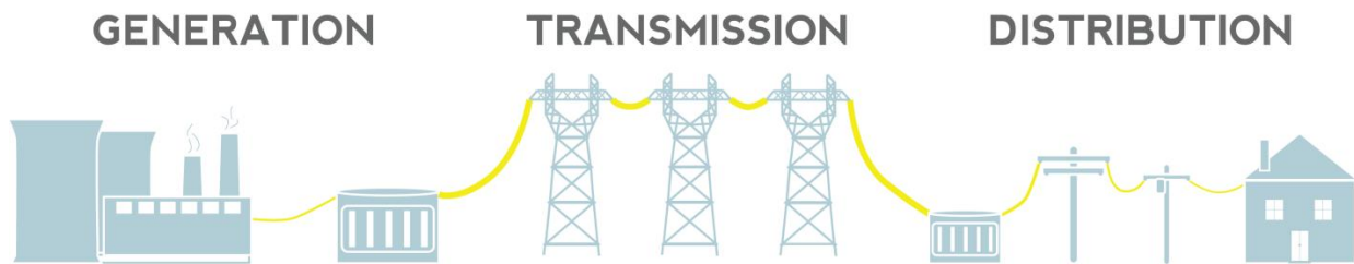
Figure 3: AC power transmission
