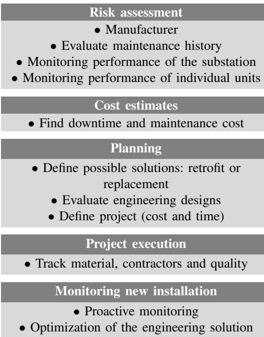
Fig. 2. Stages that are involved in the planning process of electromechanical relay replacement.
