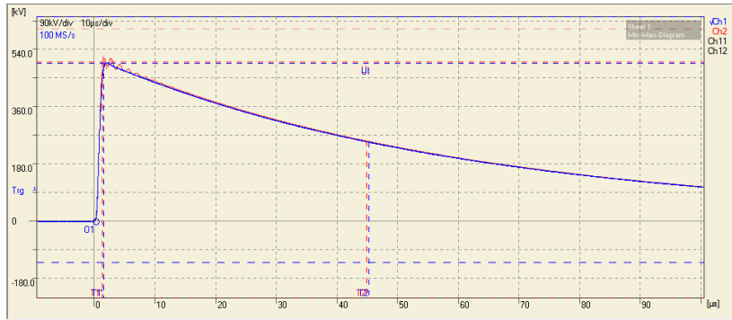
Figure 9: Lightning impulse behaviour – GIS type RGK 400DC [11]
